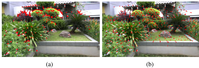
Fig. 1. Comparison of two feature point suppression approaches. (a) Using only the corner response results in few dense regions; whereas (b) using a regular grid and the corner response leads to a more uniform feature point distribution that is desirable when matching across very different viewpoints and scales.
